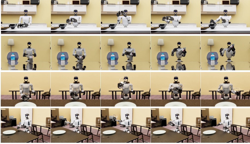
Figure A2: Robot interacts with the scene generated by SCENEWEAVER in simulation. The first three rows show the sequences of interaction in the front view in three different scenes including kitchen, meeting room and restaurant. And the last row shows the side view of the third row. Note the system keeps different materials, such as table in the meeting room has transparent and reflective material.
